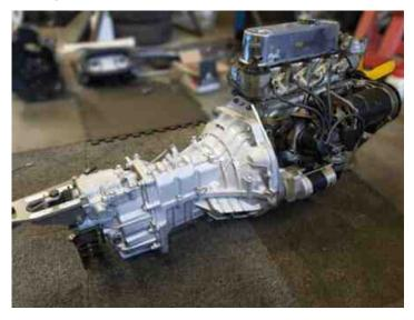
Additionally, the Jimny gearbox does not require the removal of the second cross member, a modification necessary for the T50 and T9 conversions. This makes the installation process simpler and less invasive, preserving the structural integrity of your Spridget.
